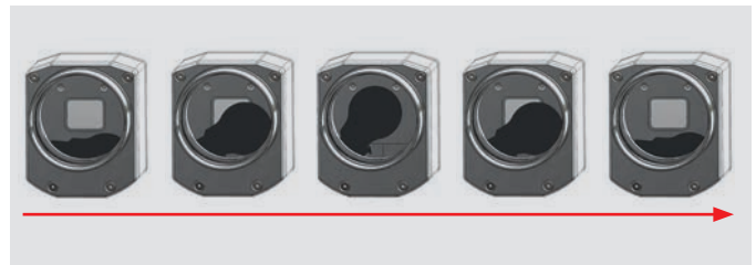
For offset referencing, a temperature reference is briefly moved into the field of view of the infrared sensor array.
