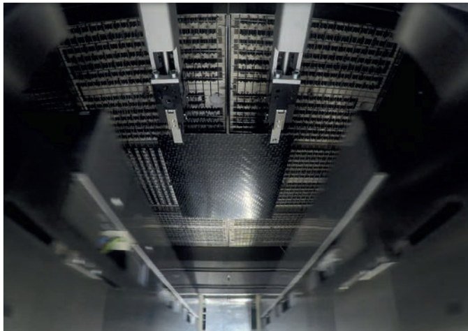
CT LT - Measuring head with laminar air purge device in a thermoforming machine
